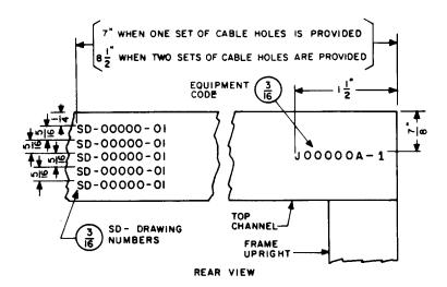
Fig. 1—Frame Equipment Code and SD- Drawing Numbers
