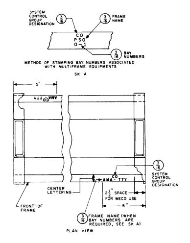
Fig. 2—Frame Name, Bay Number, and System Control Group Designations on Frame Base—Single or Multibay Sheet Metal Frame
