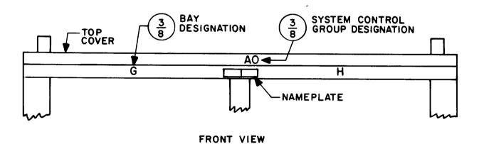
Fig. 3—Method of Stamping Frame Name, Bay, and System Control Group Designations
