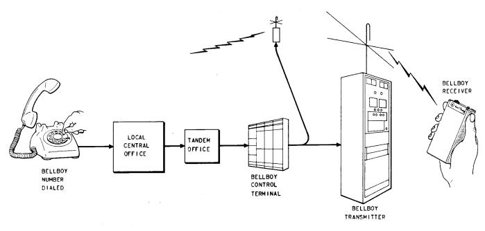
Fig. 1---Typical Setup for a BELLBOY Call
