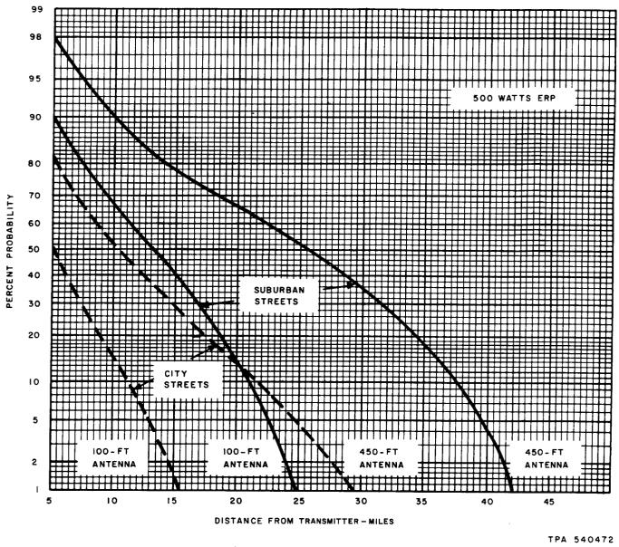
Fig. 8-Probability of Signaling a 150-MHz BELLBOY Receiver in Streets
