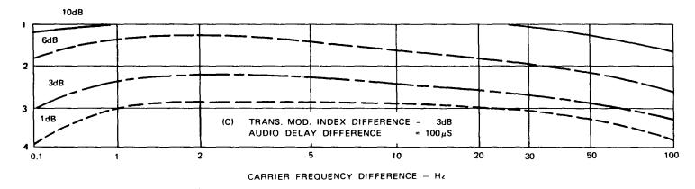
Fig. 1—Subjective Evaluation of Speech Degradation Resulting From Presence of Two Signals at Receiver Input
