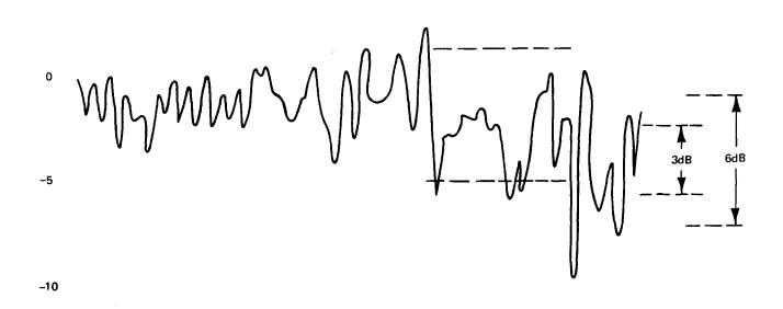
Fig. 2—Variation of 152-MHz Signal Level Along Street in Relatively Level Area
