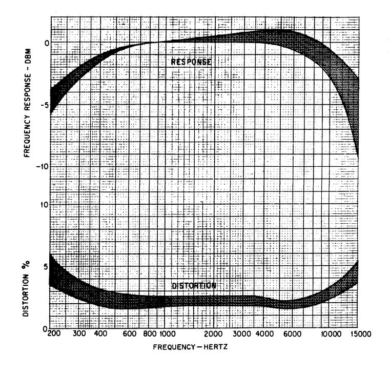
Fig. 6 — Typical Frequency Response and Distortion Characteristics GECo RC718 and DuMont MCA 474/484B Equipment
