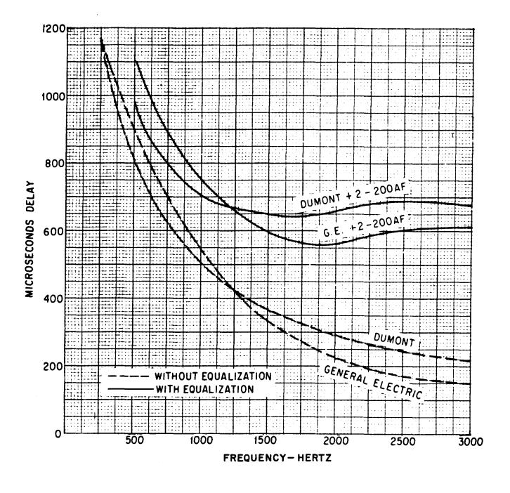
Fig. 7 — Envelope Delay Distortion — GE Single-Channel Equipment — DuMont MCA 474/484B Equipment
