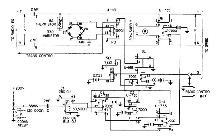
Fig. 5 – Typical Control Circuit – Connects Single-Channel Radio to 20-Hertz Ringdown Toll Line Switchboard Circuit --- Provides Signaling by **Carrier** Control
