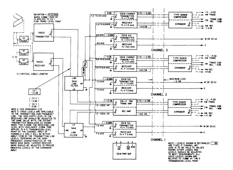
Fig. 1 — Block Diagram Showing Transmission Levels — Three-Channel Compandored System with 2- or 4-Wire Voice-Frequency Extensions with E & M Lead or Ringdown Signaling
