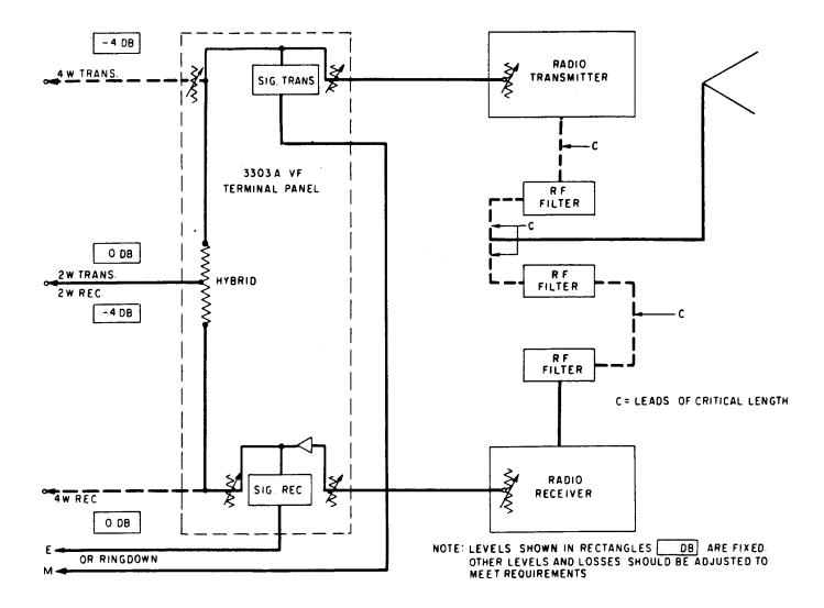
Fig. 3 — Block Diagram Showing Transmission Levels — Single-Channel Noncompandored System with 2- or 4-Wire Extensions and E & M Lead or Ringdown Signaling
