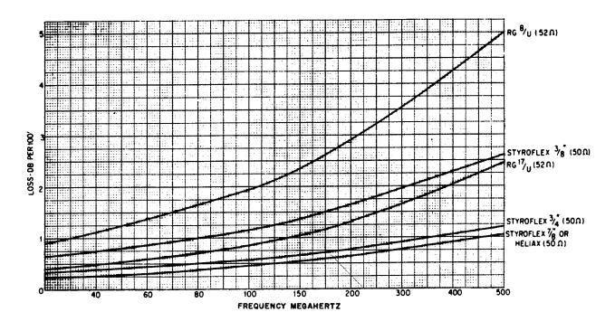
Fig. 8 — Approximate Loss of Common Types of Transmission Lines
