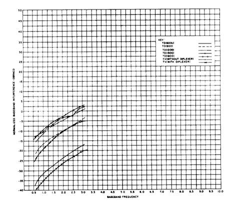
Fig. 6—Baseband Interference Into TD (600U)—20-MHz Separation
