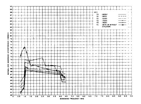
Fig. 2—Baseband Interference Into TD (900)—Cochannel Separation
