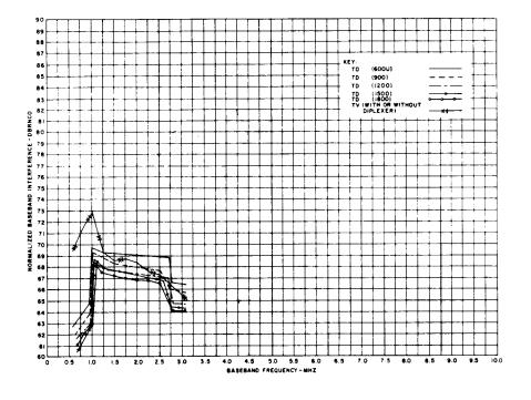
Fig. 1—Baseband Interference Into TD (600U)—Cochannel Separation
