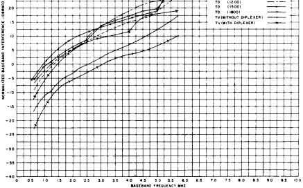
Fig. 8—Baseband Interference Into TD (1200)—20-MHz Separation
