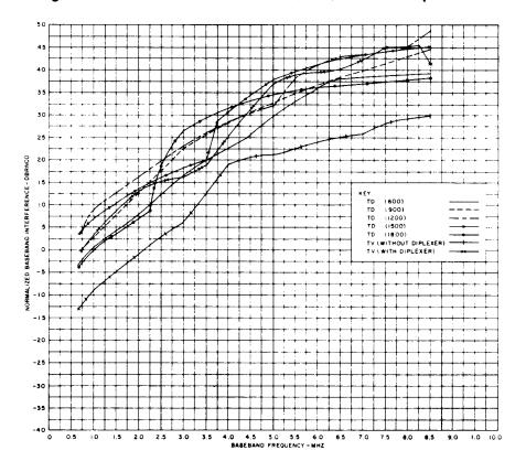
Fig. 10—Baseband Interference Into TD (1800)—20-MHz Separation
