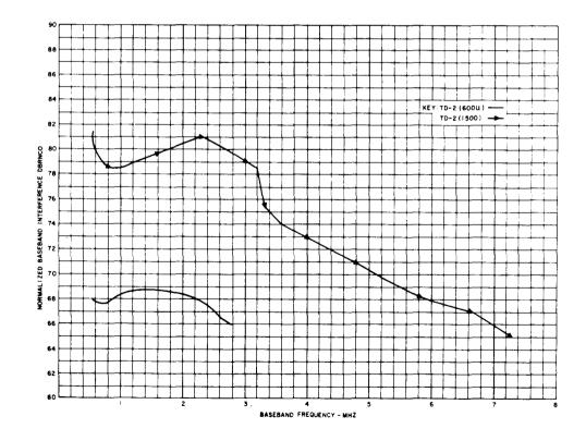
Fig. 12—Baseband Interference from TD (600L) Into TD (600U) and TD (1500)—Cochannel Separation
