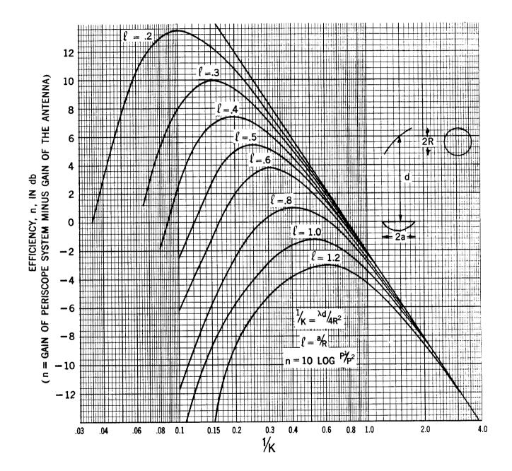
Fig. 4 – Efficiency of Periscope Antenna System Employing Curved Reflector
