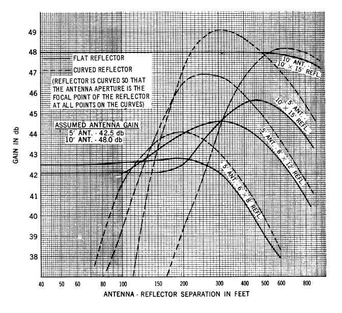
Fig. 10 – Antenna-Reflector Combinations Theoretical Gain Over an Isotropic Antenna at 11,200 Mc
