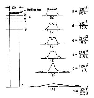
CROSS SECTIONS OF FIELD INTENSITY BENEATH A REFLECTOR
