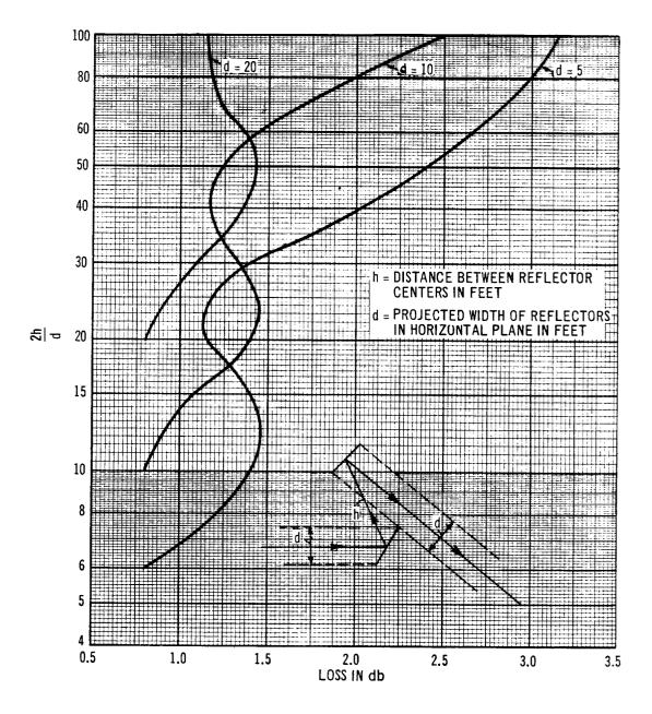
Fig. 20 – Transmission Loss From Double Reflection With Passive Repeaters
