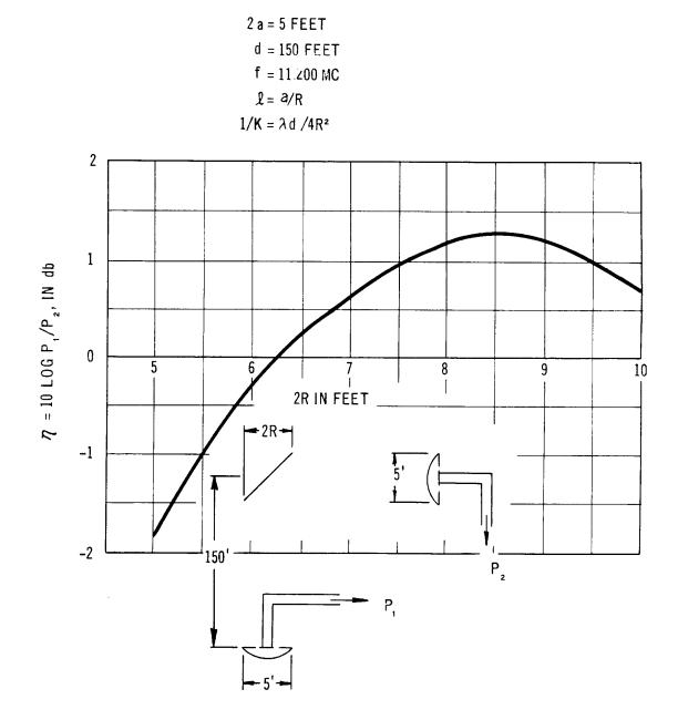
Fig. 7 – Antenna-Reflector Efficiency v. Reflector Size
