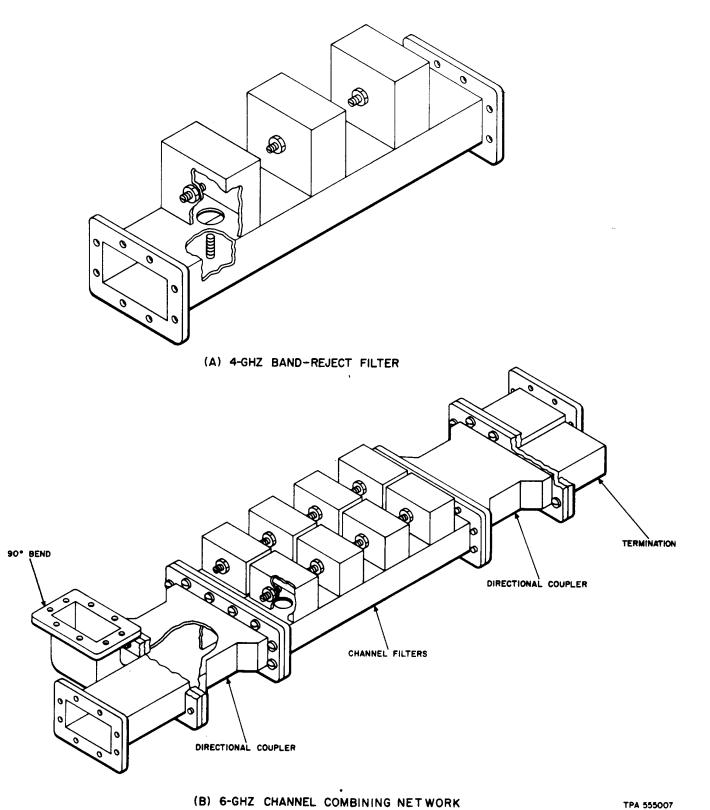
Fig. 2—Examples of Waveguide Type Circuit Components
