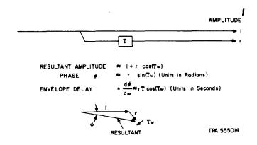
Fig. 9-Approximate Delay Characteristic
