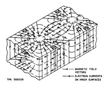
Fig. 4—Surface Current in Rectangular Waveguide
