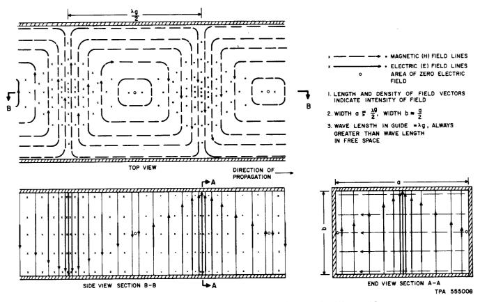
Fig. 3—Relative Fields in Dominant Mode Rectangular Waveguide
