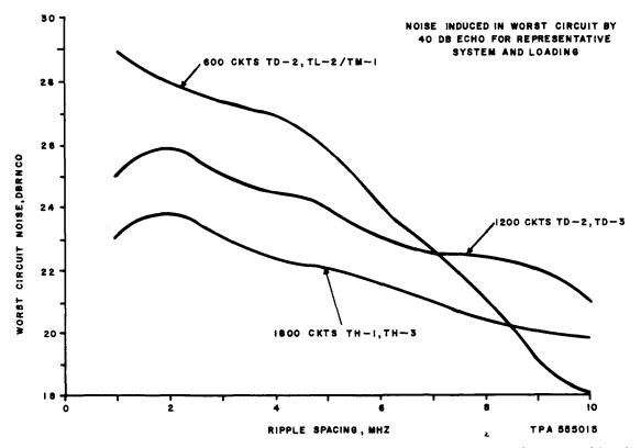
Fig. 10—Noise Induced in Worst Circuit by 40-dB Echo for Representative System and Loading
