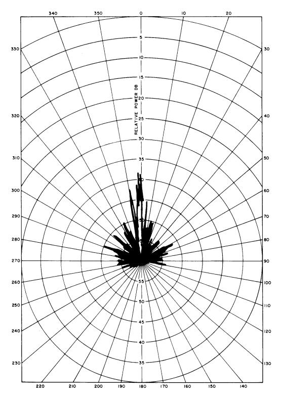
Fig. 7—Response to Cross-Polarized 6.175 GHz Signal
