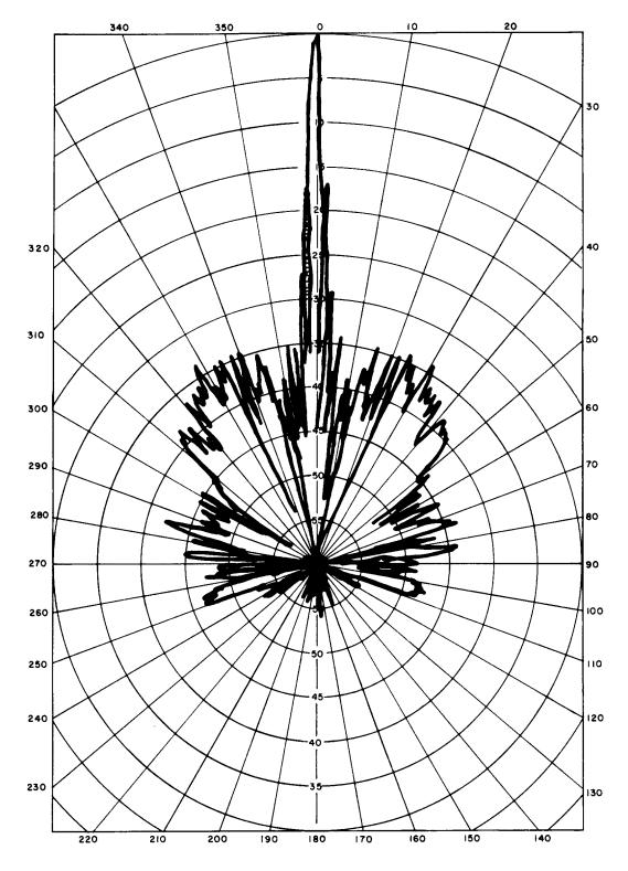
Fig. 4—Radiation Pattern for Vertically Polarized 6.175 GHz Signal
