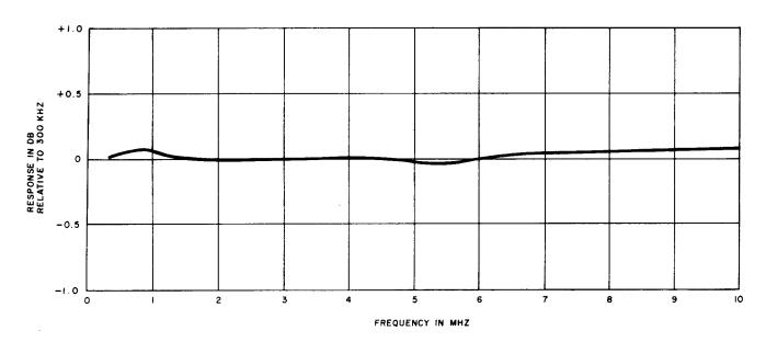
Fig. 6—TH-1 FM Terminal Pair Baseband Response
