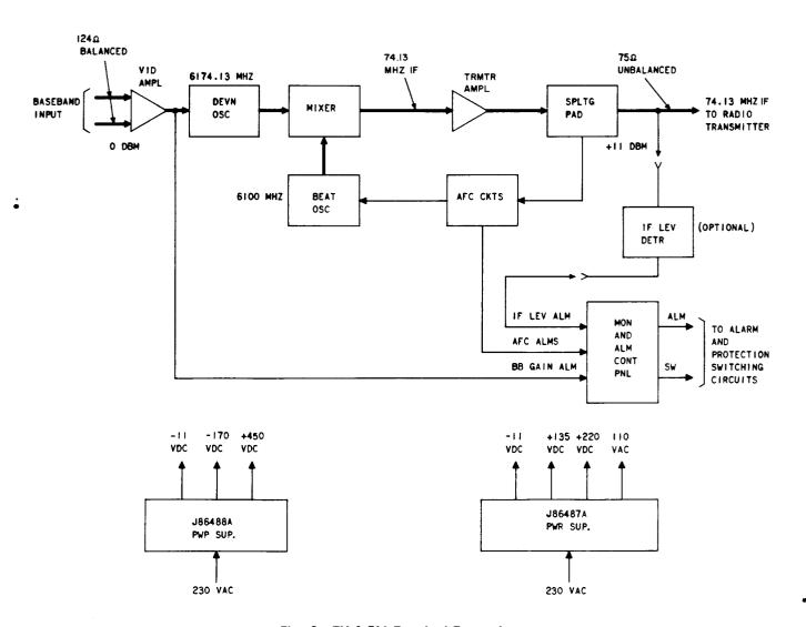
Fig. 2—TH-1 FM Terminal Transmitter
