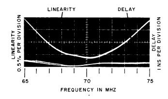
Fig. 9—3A/4A FM Terminal Pair Linearity and Delay
