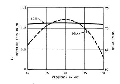
Fig. 3—4167A Network Delay and Insertion Loss
