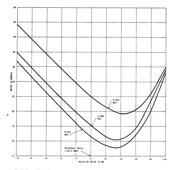
Fig. 5—Typical 3A/4A FM Terminal Pair 1800-Circuit Noise Load Curves (With 457D and 457E Networks)
