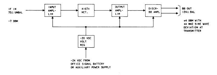
Fig. 2-4 FM Terminal Receiver Block Diagram
