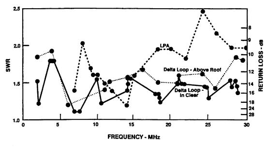
Fig. 4 - Measured Standing-Wave Ratios of Three Antennas
