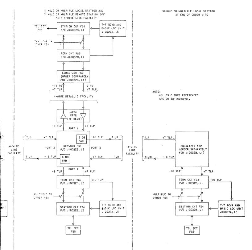
Fig. 2—Typical Equipment Combinations and Transmission Interfaces for Single Order Wire
