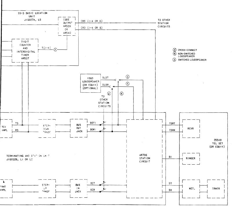
Fig. 4—Block Diagram of Single Line-Single Station Units
