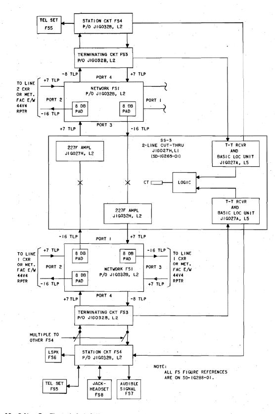
Fig. 10—2-Line Cut-Through Switch Installation—With Terminating and Station Equipment on Both Lines
