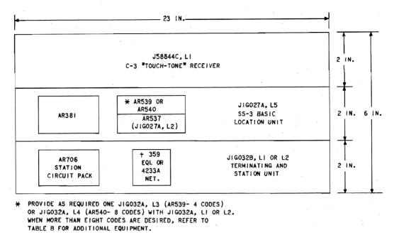
+ WHEN JIG032B, LI IS PROVIDED, 359-TYPE EQUALIZER MUST BE ORDERED SEPARATELY. NETWORK 4233A IS PROVIDED WITH JIG032B, L2.
