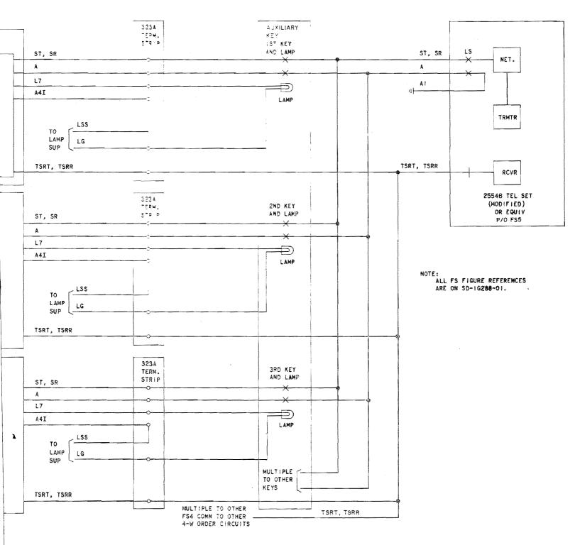
Fig. 6—Block Diagram of Multiple Line-Single Station Arrangement
