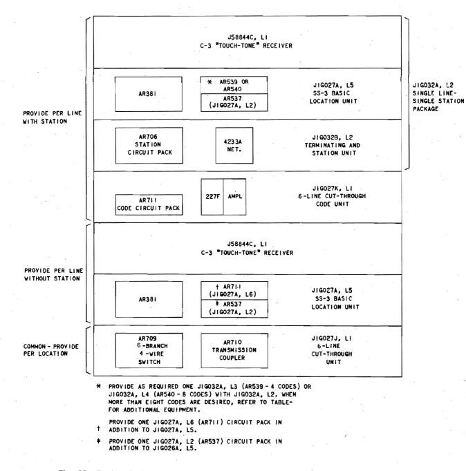
Fig. 11—Typical Equipment Arrangement for 2- to 6-Line Cut-Through Switch Installation
