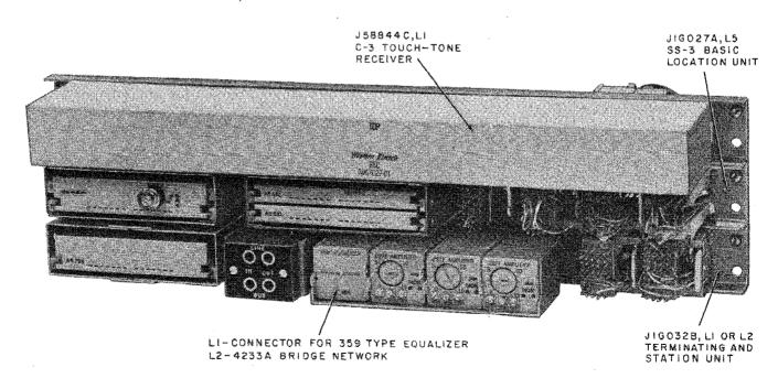
Fig. 1—Single Line-Single Station Packaged Units J1G032A, L1 or L2
