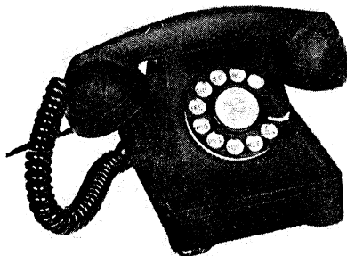
Fig. 1 — 304-type Telephone Set
