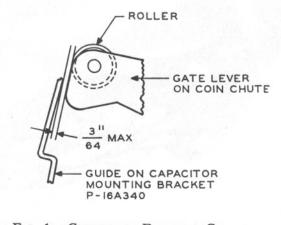
FIG. 1—CLEARANCE BETWEEN GUIDE AND GATE OPERATING ARM gong and is at right angles to face of gong mounting bracket. Judge visually. Handset-type coin collectors shall be equipped with oval-type gongs. Final judgment of signal tones should be determined by coin signal tests with the operator as called for in the C Section covering prepay or postpay maintenance. If satisfactory signals are not obtained, upper housing shall be replaced.
