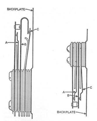
MIN. 1/32" CLEARANCE BETWEEN SPRINGS A AND B, AND BETWEEN SPRING C AND BACKPLATE.JUDGE VISUALLY.
