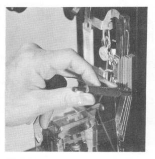
FIG. 6—Adjustment of Housing Contact Springs
