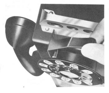
FIG. 2—METHOD OF INSTALLING P-14A544 COIN DEFLECTOR
