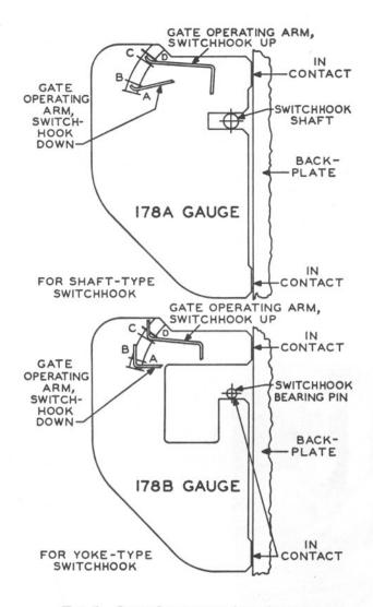
FIG. 5-GATE OPERATING ARM ASSEMBLY
