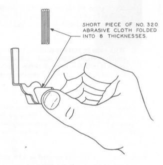
Fig. 9 - Polishing of Fork Slot
