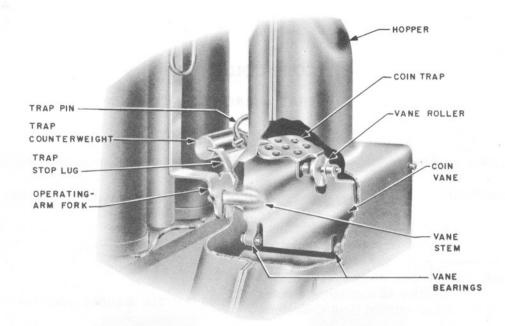
Fig. 2 - Hopper and Rear of Coin Relay
