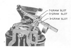
Fig. 3 - Gauge for Ground Spring Contact Force
