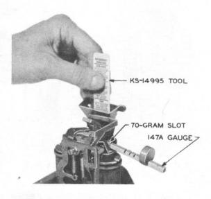
Fig. 7 — Trap and Vane Release Test
