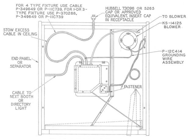
Fig. 6 — Typical Installation for 3-way Receptacle
