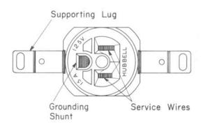
Fig. 4 — Hubbell No. 5261, 3-wire Grounding-type Convenience Outlet
