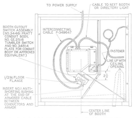
Fig. 9 - Typical Cutout Switch Installation with 4-type Light Fixture
