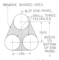
Fig. 12 - Hole for 2D Fixture
