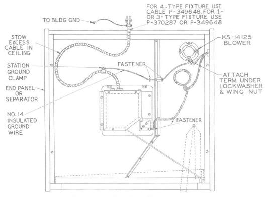
Fig. 8 - Typical 2-wire Cable Arrangement
