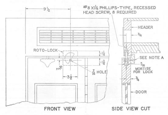
Note: Replace P-381074 (1-1/2 inch) door stop screws with 1-inch wood screws (three required).
