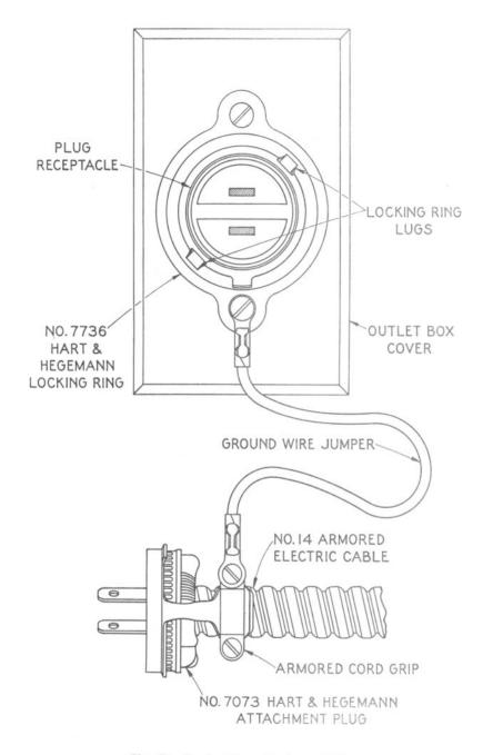
Fig. 7 - 2-wire Receptacle and Plug
