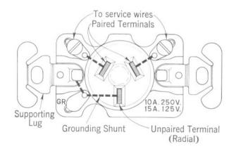
Fig. 3 – 3-wire Flush-type Receptacle with Grounding Shunt
