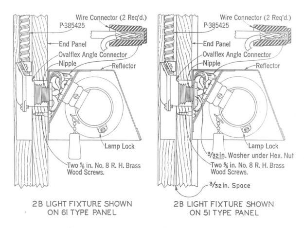
Fig. 13 — Installation of 2-type Light Fixture
