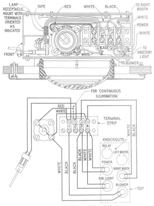
Fig. 11 — 4A Light Fixture for Four Cables
