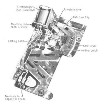
Fig. 10 — Prepayment Steel Coin Chute — with Cutover Clip for 5¢ Service
