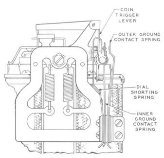
Fig. 11—3-spring (Dial Shorting) Relay— Contact Spring Guard Cut Away
