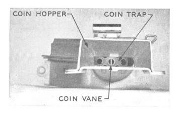
Fig. 9 — Position of Vane when Relay is Centered
