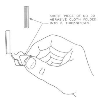
Fig. 8 - Polishing of Fork Slot
