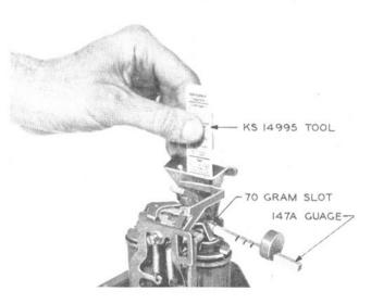
FIG. 4 - TRAP AND VANE RELEASE TEST
