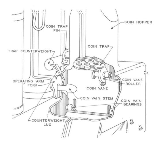
FIG. 2 - COIN HOPPER AND REAR OF COIN RELAY
