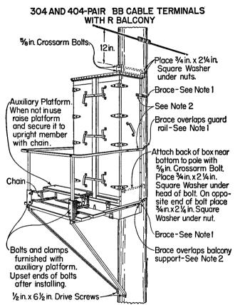
Note 1- Fasten to pole with ½ in. x 4½ in. Drive Screw. Note 2- ¾ in. x 2½ in. Carriage Bolt. Place ‰ in. x 1¾ in. Round Washer under head of bolt inside Terminal.
