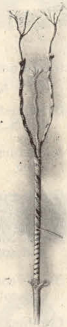
Method of Stranding Tinsel Switchboard Cord
